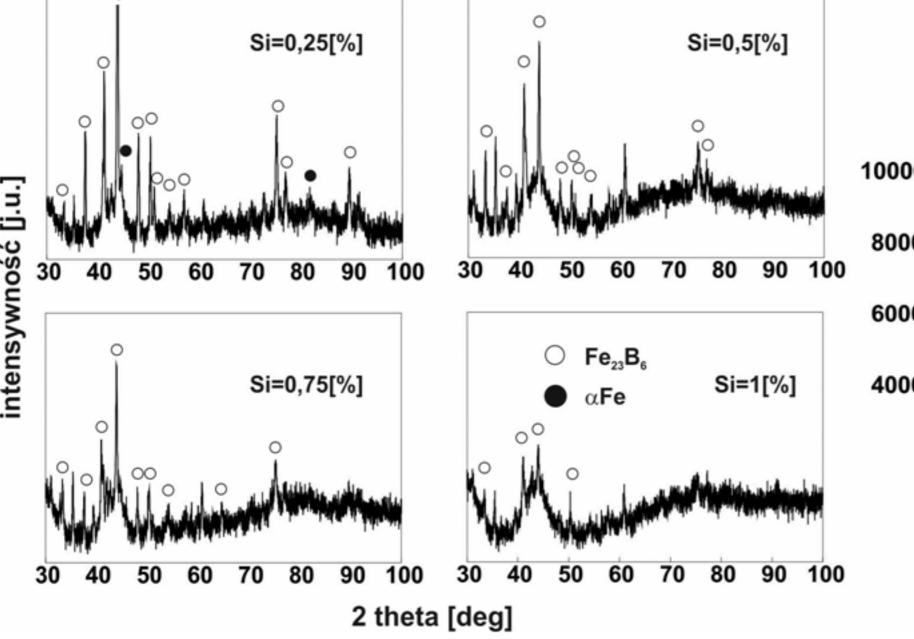
A nanocrystalline massive iron alloy characterized in that it has the atomic composition of Fe65Co11-xB20SixZr2Hf2, where the value of x is 0.25 or 0.5 or 0.75 or 1, and the permissible amount of impurities does not exceed 0.09%.
