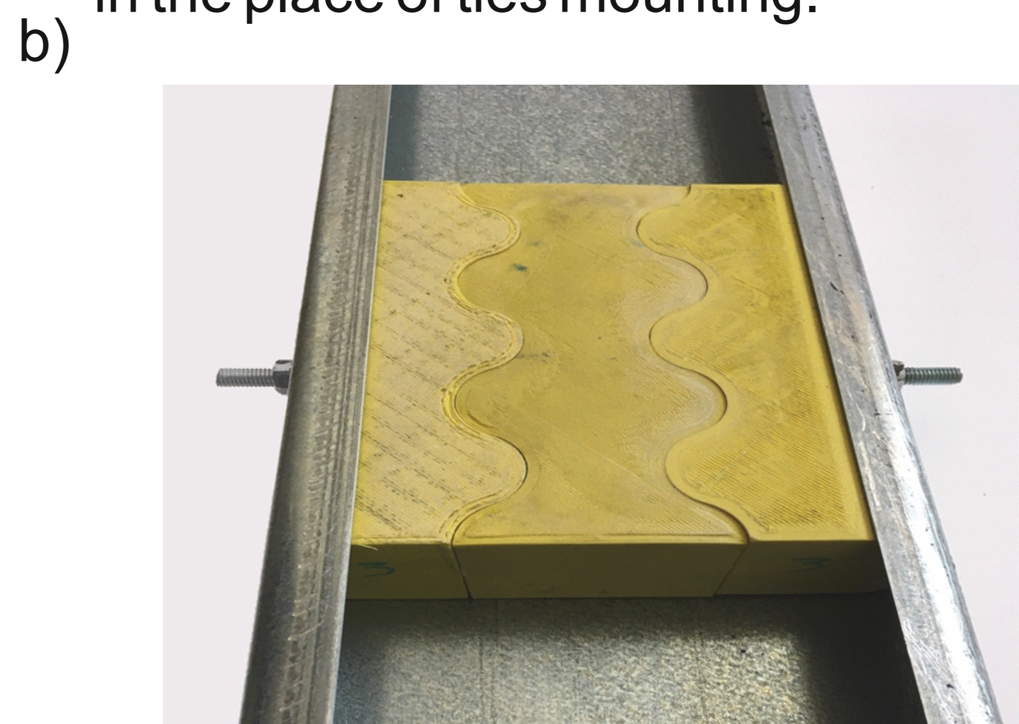
Fig.2. Stiffening insert, preferably of thin-walled C-type sections: a) view of the three elements forming the stiffener, b) view of the stiffener in the thin-walled profile.
