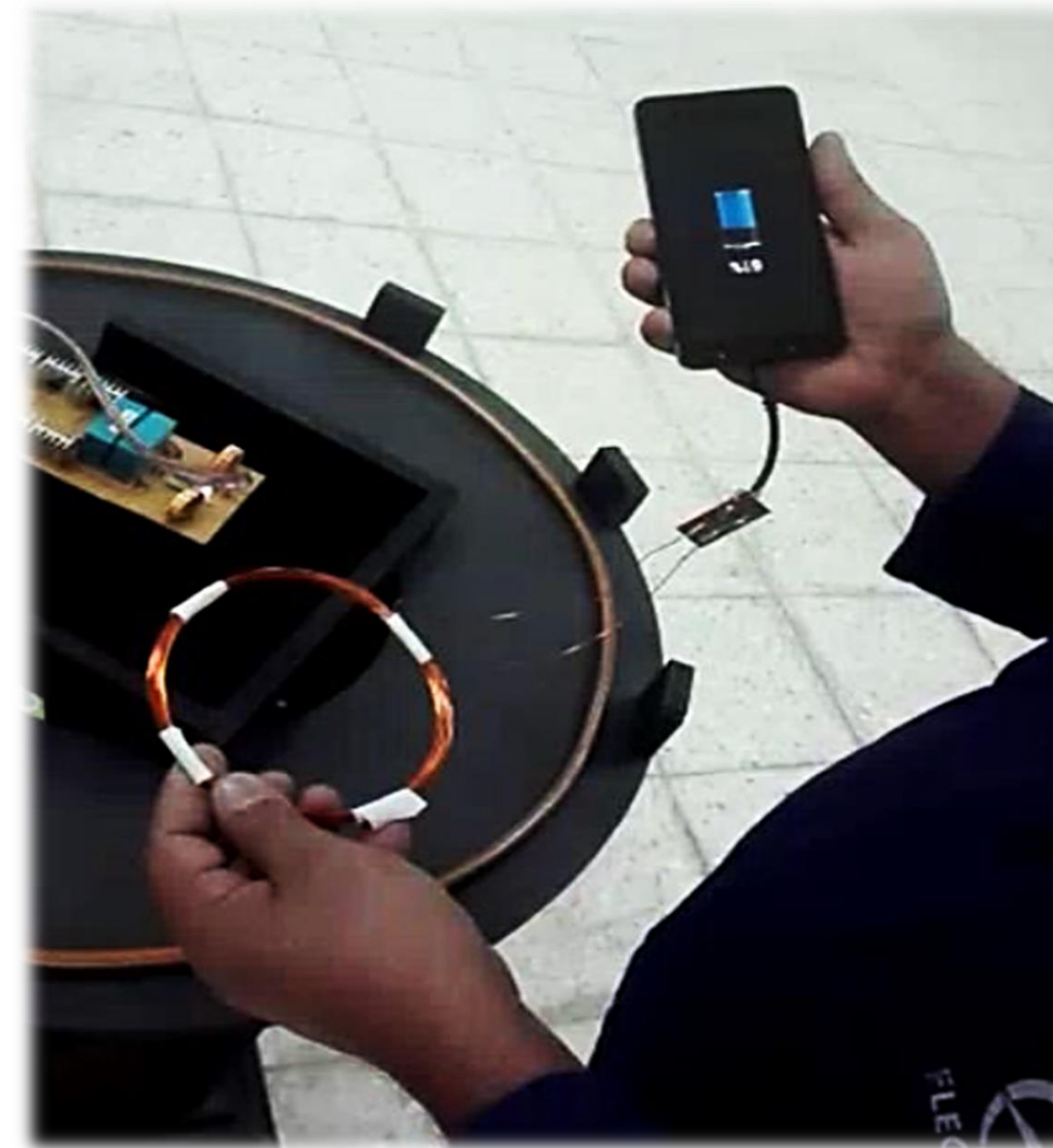
Fig (1): A mobile phone charging from a distance away from the transmitter
