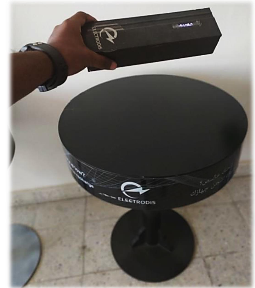
Fig (2): Wireless laptop/mobile device charging café table and its concept photo
