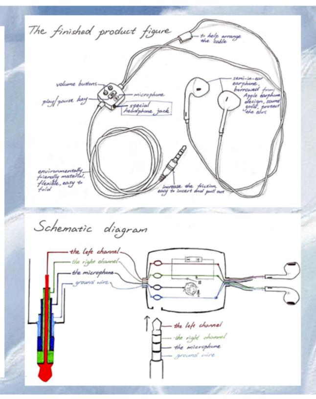
A common earphone has four lines: left channel, right channel, microphone and ground. Our idea is to place four special metal rings on each of the four lines corresponding to the earphone jack. In this way, when the other earphone is inserted, it can be combined with each metal ring to share information with the inserted earphone. That's how we made it possible for music to be shared by multiple people using multiple earphones by adding a headphone jack to a normal earphone.
