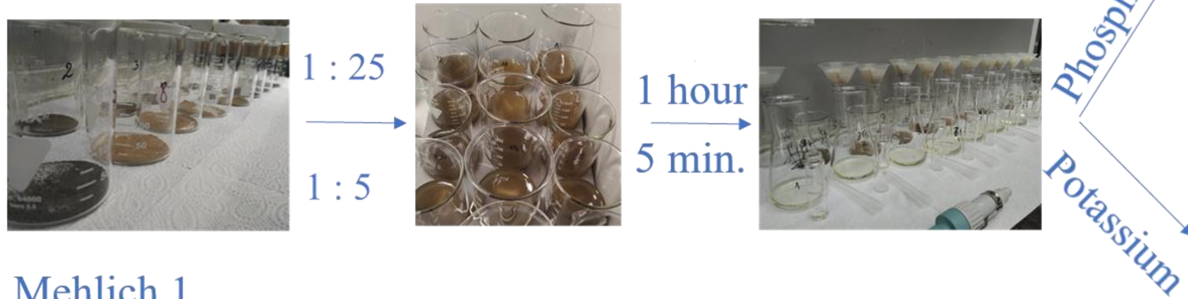
Figure 2: Schematic representation of Mehlich 1 and Acetate-lactate method (Ivanov) for extraction and determination of K and P in soil samples.
