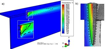
Temperature distribution in T-joint: a) temperature profile, b) comparison of temperature distribution in the cross section of the joint with the real weld.
