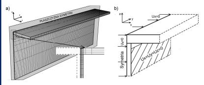
In order to reduce computational time, symmetry of the joint is assumed in calculations taking into account appropriate boundary conditions in the plane of symmetry.
