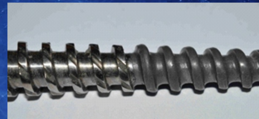
Screw of extrusion machine partially coated by polymer-powder slurry
