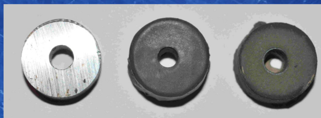
Sample of unalloyed steel, a) uncoated, b) coated, c) sintered
