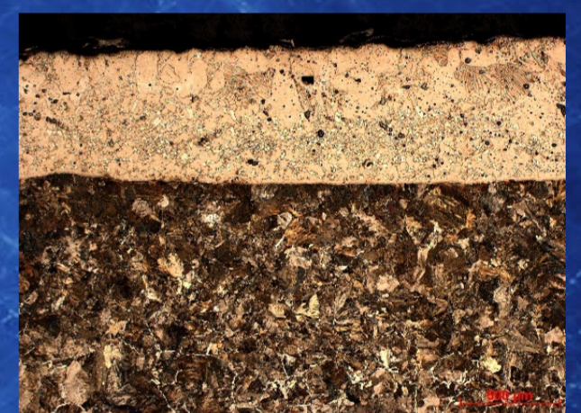
Layer of ferritic steel etched with nital
