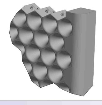
The shape of the individual panels should be such that they cover the entire surface (in the example, a regular hexagon, but you can also use squares, triangles, etc.).
