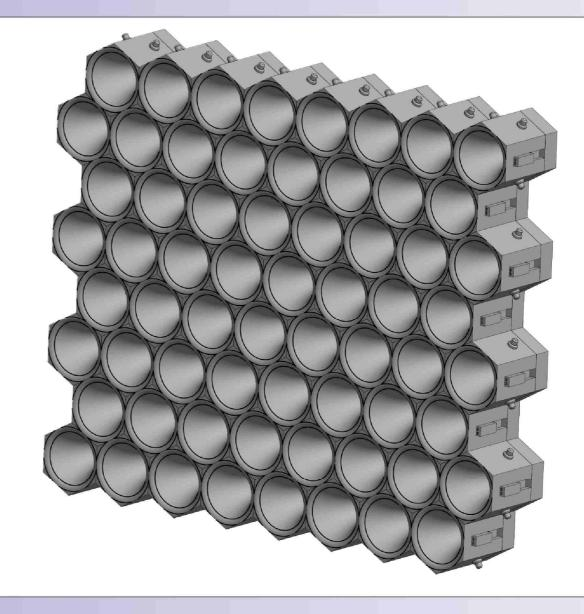
The modular construction allows the use of the invention to cover the walls of buildings, allowing to leave free space for the windows or doors.
