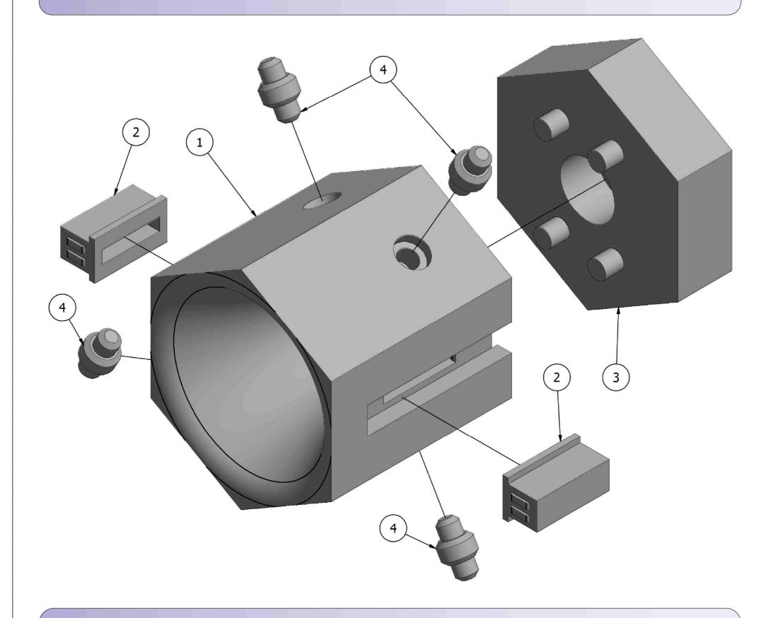
The incident wave horn type panel (1) is constructed in such a way as to intercept the incident mechanical wave and direct it to the energy harvesting module (3), which, depending on the version, converts it using piezoelectric or electromagnetic elements into electricity.
