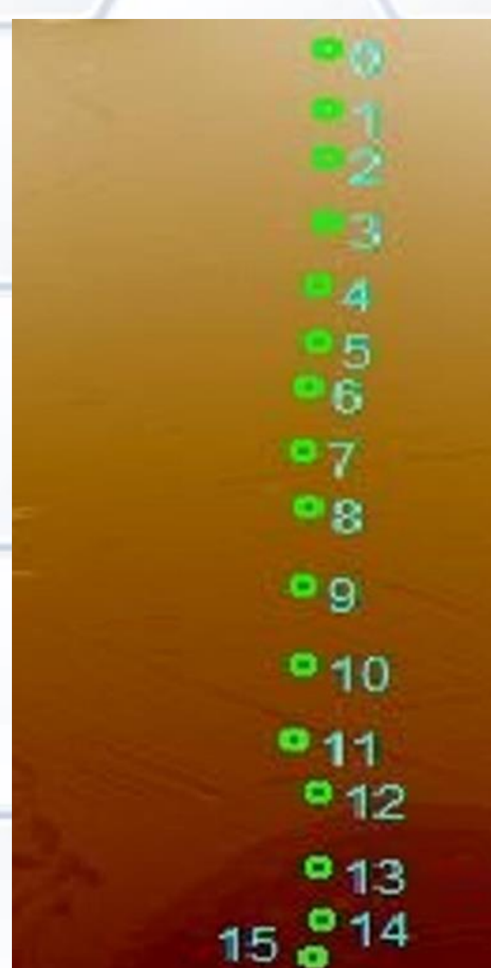
Fig 7. The predefined points across the cross-section of the shell, transition area and core used for nanoindentation measurements.
