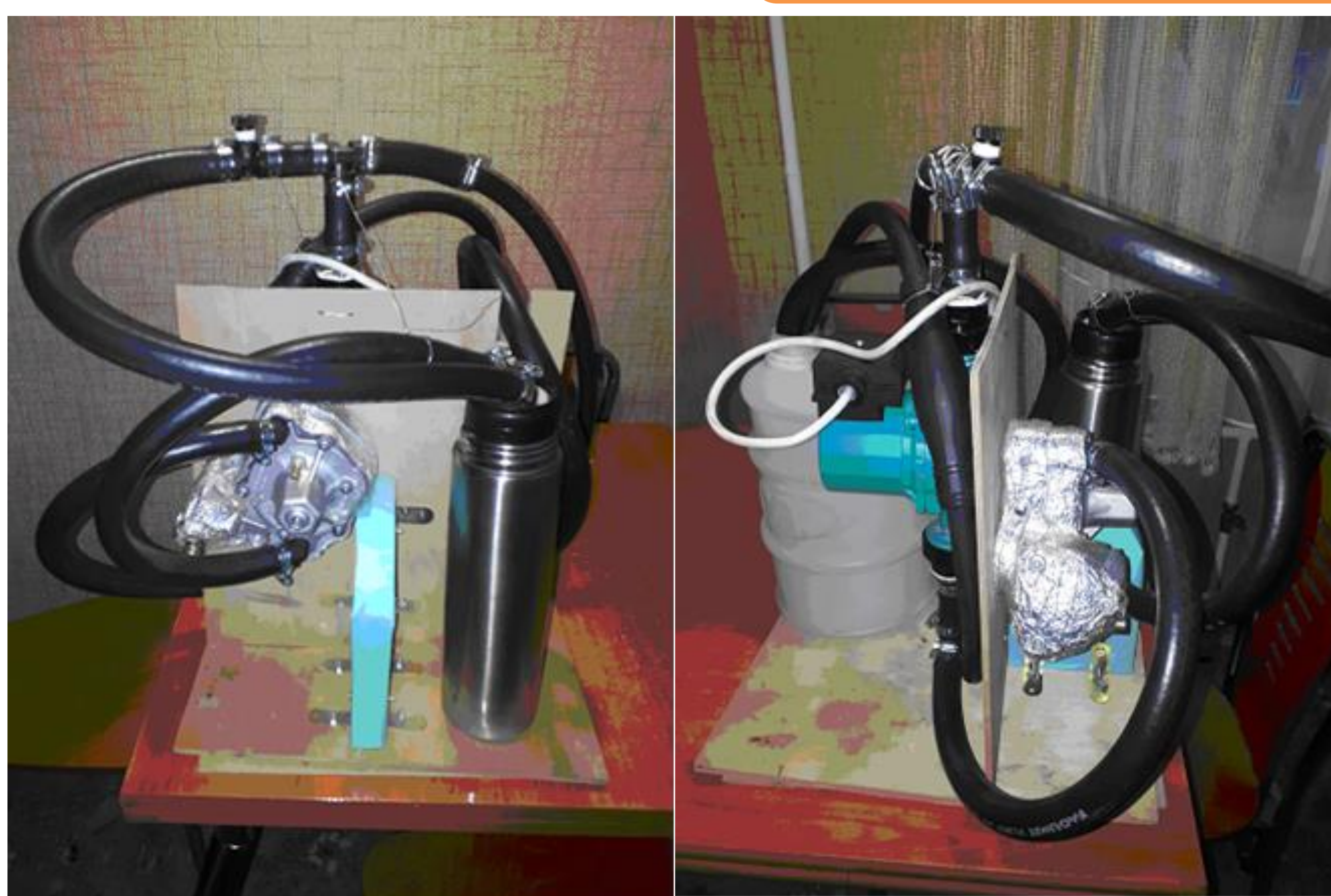
Layout of the system of fast heating of a gas reducer
