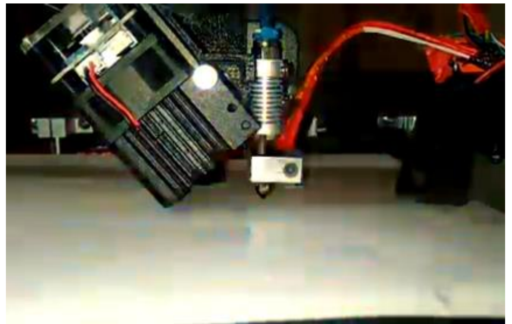
Figure 1. The 3D printer with an additional temperature regulation system
