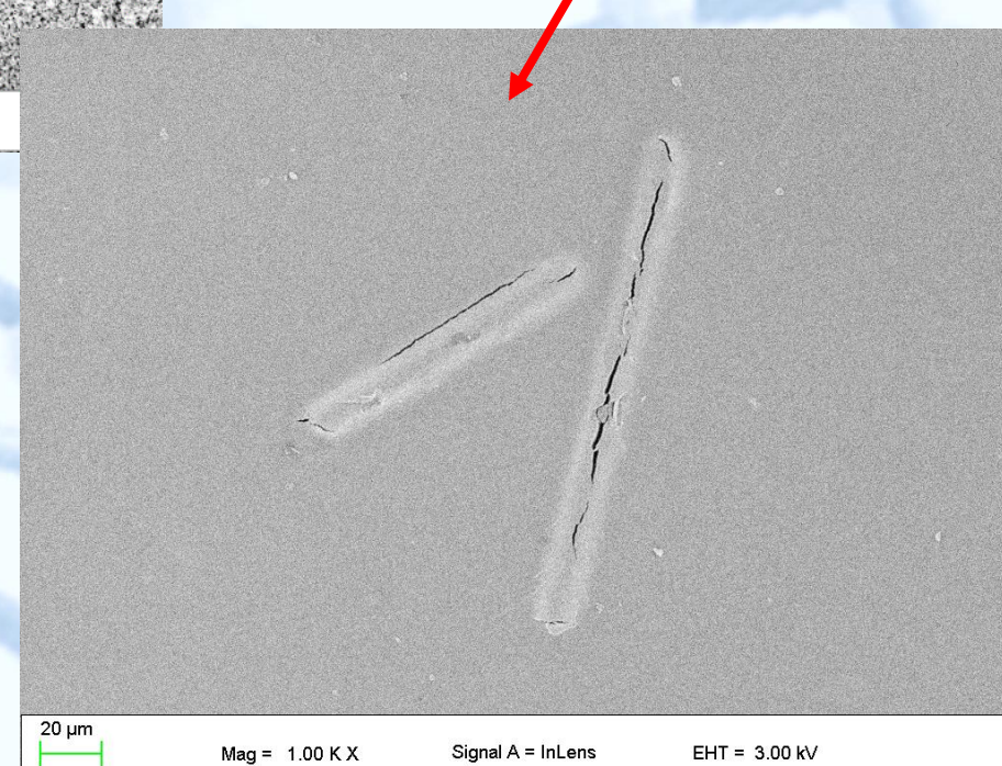
Topography of TiO 2 layer with carbon fibers
